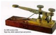
The 1848 model of the Morse key, which replaced the pen and parchment. Telegraph: Few bits per second!
